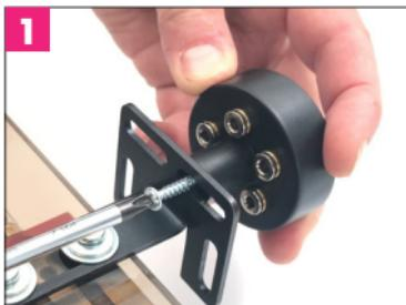
1. Attach connecting adapter SLM (Art.290-29000), connect the lubrication lines to the 5 lubrication points (see our accessories on page 14).
