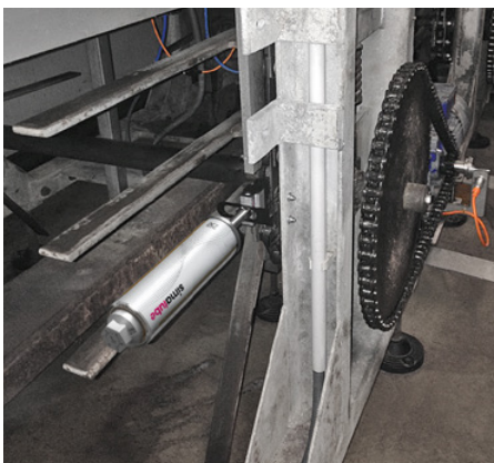
Chain lubrication with a 250 ml simalube and a flat brush.
