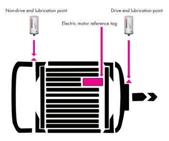
«simalube lubricates continuously, extends the service life of your electric motor and reduces maintenance costs»
