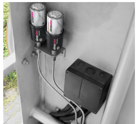
Due to permanently installed lubrication lines on a pool cleaner, two simalube IMPULSE connect are used. They overcome the back pressure and ensure continuous lubrication.
