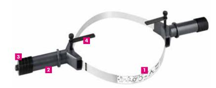
The Bearing Handling Tool is ideally suited for professionally and securely lifting large, heavy bearings. The BHT reduces the risk of accidents and bearing damage. The BHT encloses the outer race of the bearing with a steel band. With two handles on opposite sides and two carrying belts, the bearing can be easily transported with a lifting crane. The bore remains open so the bearings can be easily placed onto a shaft.
