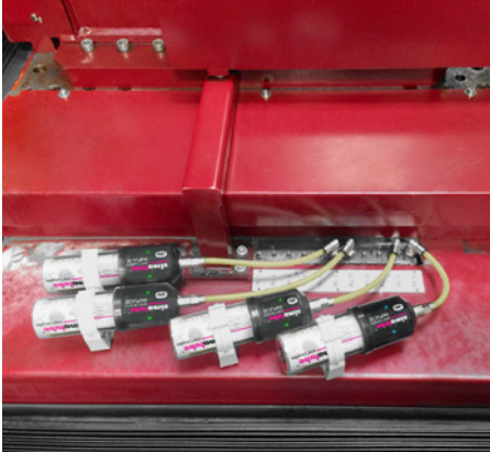
Four simalube IMPULSE connect pressure boosters lubricate the linear guides of a CNC machine by means of hose connections. Each IMPULSE can be controlled and configured individually with the simatec app.
