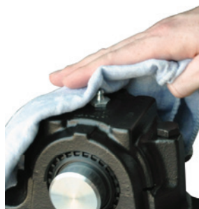
Clean lubrication point
