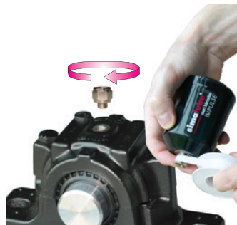
Screw in reducing nipple and seal lubrication point
