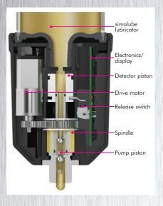
The simalube® IMPULSE ensures reliable lubrication in situations with high counterpressure and long lubrication lines. With the automatic simalube lubricators, this pressure booster pumps greases and oils at up to 10 bar and 0.5 ml per impulse to the targeted lubrication point. The LED display of the intelligent pressure booster provides information continously about the current operating condition, and flashes green when the device is functioning correctly.
